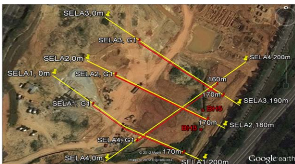
Figure 2. The survey area with survey lines and boreholes.
