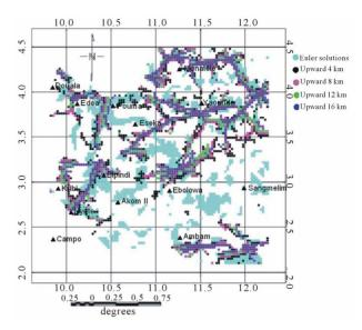
Figure 7. Estimated locations of contacts according to the horizontal gradient coupled with upward continuation method and Euler deconvolution method.
