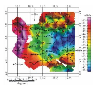
Figure 3. Bouguer anomaly map, black triangles indicate the localities and black round dots indicate gravity stations.
