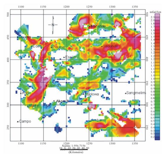
Figure 4. Horizontal gradient map of simple Bouguer anomalies.
