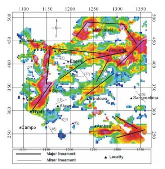
Figure 8. Gravity lineament map obtained for the study area superimposed on the horizontal gradient map.
