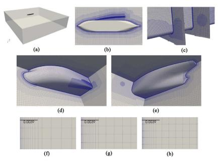
**Figure 6.** (a) Computational domain and hull; (b)-(d) Coarse mesh with refinement regions; (e)-(f) Mesh representing the hull boundary layer and the hexahedral isotropic mesh beyond. The overall layer thickness of the medium mesh is about 3.9 mm. (a) Domain; (b) View from below the hull; (c) Refinement near FSV separation (medium mesh); (d) Bow view; (e) Stern view; (f) Coarse; (g) Medium; (h) Fine.
