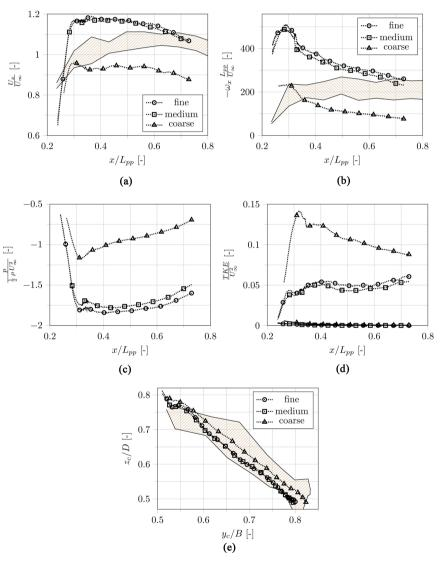
**Figure 11.** Evolution of the flow at the vortex centre and its position. The circle, square and triangle marks represent the fine, medium and coarse mesh. The shaded region between the solid lines represents the experimental results. (a) Axial velocity; (b) Axial vorticity; (c) Pressure coefficient; (d) TKE: dotted-resolved, solid-modelled; (e) Vortex centre position. FSV separates in top left corner.
