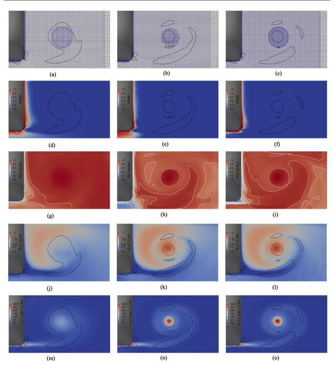
**Figure 9.** Different flow fields at  $x/L_{pp} = 0.6$  (near A-A in **Figure 1(a)**) based on **time-averaged** fields for the three meshes: left-coarse, centre-medium, right-fine. Black isolines represent  $QL_{pp}^2/U_{\infty}^2 = 22.6$ , white isolines represent TKE resolved by total in steps of 0.1. (a)-(c) mesh; (d)-(f) blending between LES and RANS; (g)-(i) resolved TKE to total TKE; (j)-(l) axial velocity; (m)-(o) axial vorticity.
