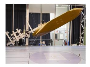
Figure 4. Model and PIV system in the test section.
