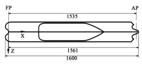
**Figure 2.** Side view of KVLCC2 as double body model with forward perpendicular (FP), after perpendicular (AP),  $L_{oa}$ ,  $L_{pp}$  and distance between transom stern and FP (in [mm]). The origin of the coordinate system is placed in the intersection of the forward perpendicular and the double-body symmetry plane or the waterline.
