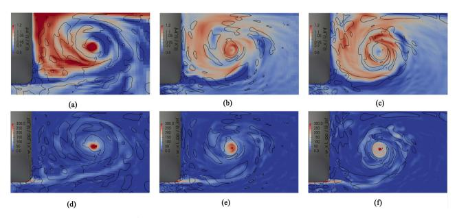
**Figure 10.** Different flow fields at  $x/L_{pp} = 0.6$  (near A-A in **Figure 1(a)**) based on instantaneous fields for the three meshes: left-coarse, centre-medium, right-fine. Black isolines represent  $QL_{pp}^2/U_{\infty}^2 = 22.6$ . (a)-(c) axial velocity; (d)-(f) axial vorticity.
