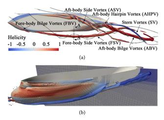
**Figure 1.** KVLCC2 at 30° drift angle with vortices. Isosurfaces both coloured by normalized helicity. (a) Qualitative view of the vortex system and selected streamlines. The plane A-A indicates an exemplary measuring plane for the analysis of the FSV; (b) Evolution of the FSV on the medium mesh with isosurface  $QL_{pp}^2/U_{\infty}^2 = 100$  (based on time-averaged flow). The plane showing the mesh is near A-A in subfigure (a).
