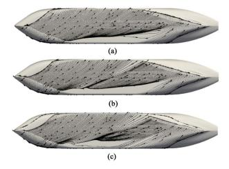
**Figure 12.** Limiting streamlines based on time-averaged wall shear stress. Streamlines are based on the same seeding line along the *x*-axis on the hull's bottom. (a) Coarse; (b) Medium; (c) Fine.
