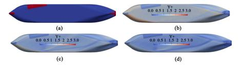
**Figure 7.** Near wall mesh resolution, dimensionless wall distance  $Y^+$  based on timeaveraged flow. Small  $Y^+$  values correspond to small cell sizes on the hull. (a) Cell level at the hull, blue-level 6, red-level 7; (b) Coarse; (c) Medium; (d) Fine.
