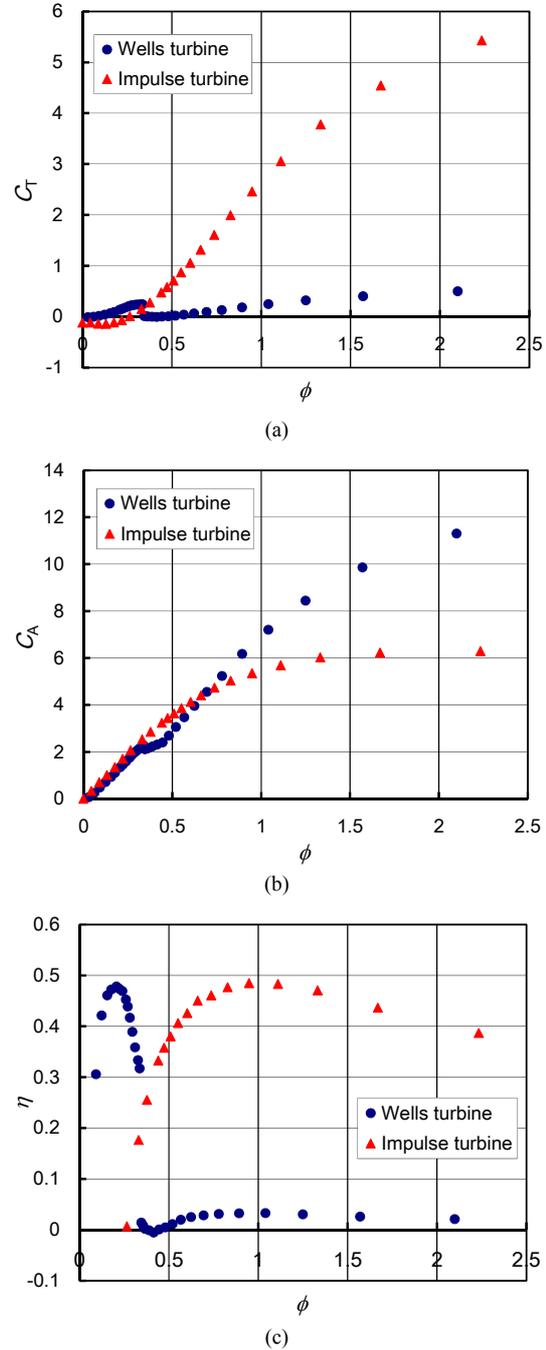
**Figure 7. Turbine characteristics under steady flow conditions: (a) Torque coefficient; (b) Input coefficient; (c) Efficiency.**
