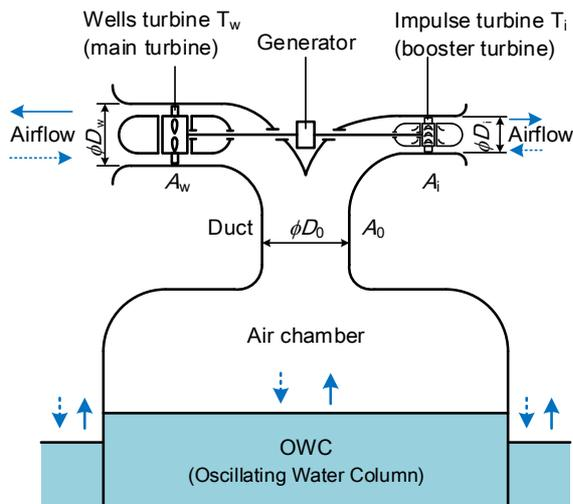
Figure 3. Principle of plant using Wells turbine with booster turbine.
