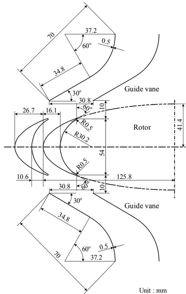
**Figure 6. Tested impulse turbine ( $D_i = 300$  mm).**
