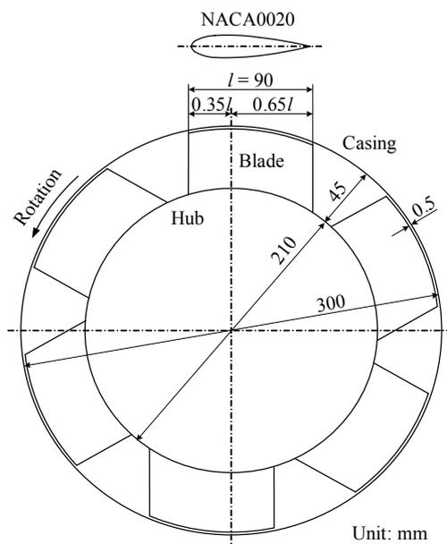
**Figure 5. Tested Wells turbine ( $D_w = 300$  mm).**
