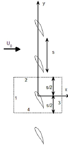
**Figure 1. Control volume for cascade of equi-spaced identical bodies.**
