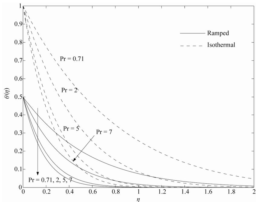
Figure 8. Temperature profiles for variations in Pr when Ra = 2 and tau = 0.5 .
