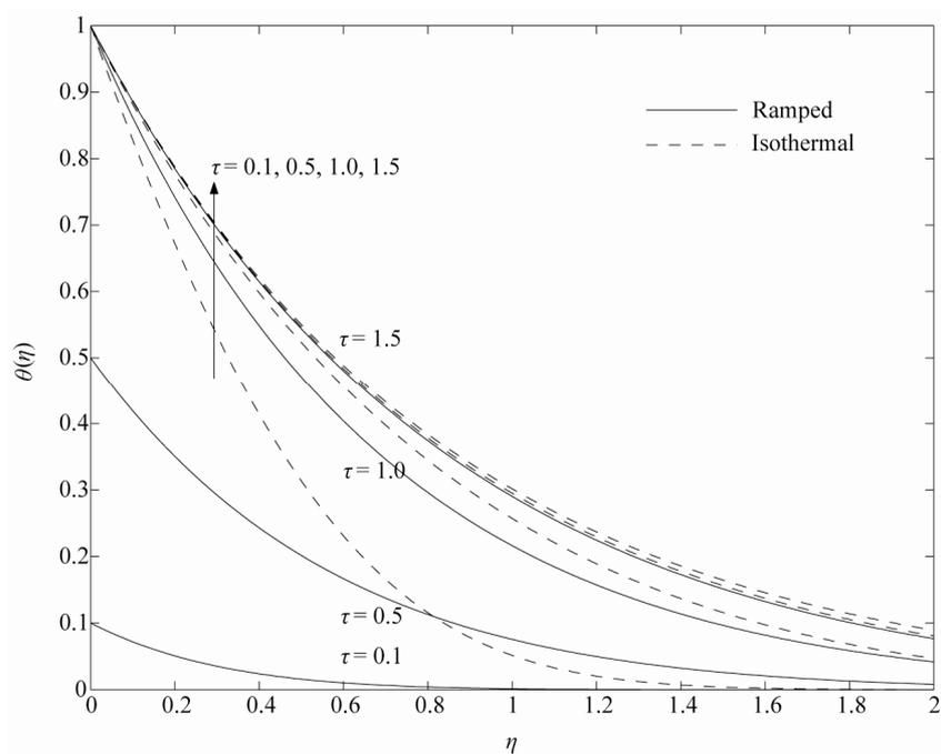
Figure 9. Temperature profiles for variations in time tau when Pr = 0.71 and Ra = 2 .
