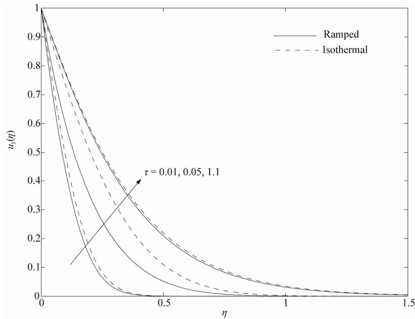
Figure 6. Velocity profiles for variations in time  $\tau$  when  $Pr = 0.71$ ,  $Gr = 25$ ,  $Ra = 2$  and  $Da = 0.04$ .
