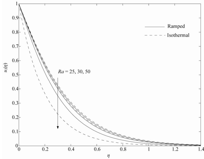
Figure 2. Velocity profiles for variations in  $Ra$  when  $Pr = 0.71$ ,  $Gr = 25$ ,  $\tau = 0.1$  and  $Da = 0.04$ .
