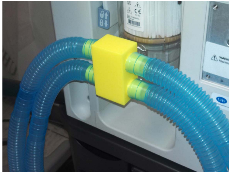
Figure 2. “Fit” Test of 4-port manifold on Ventilator.
