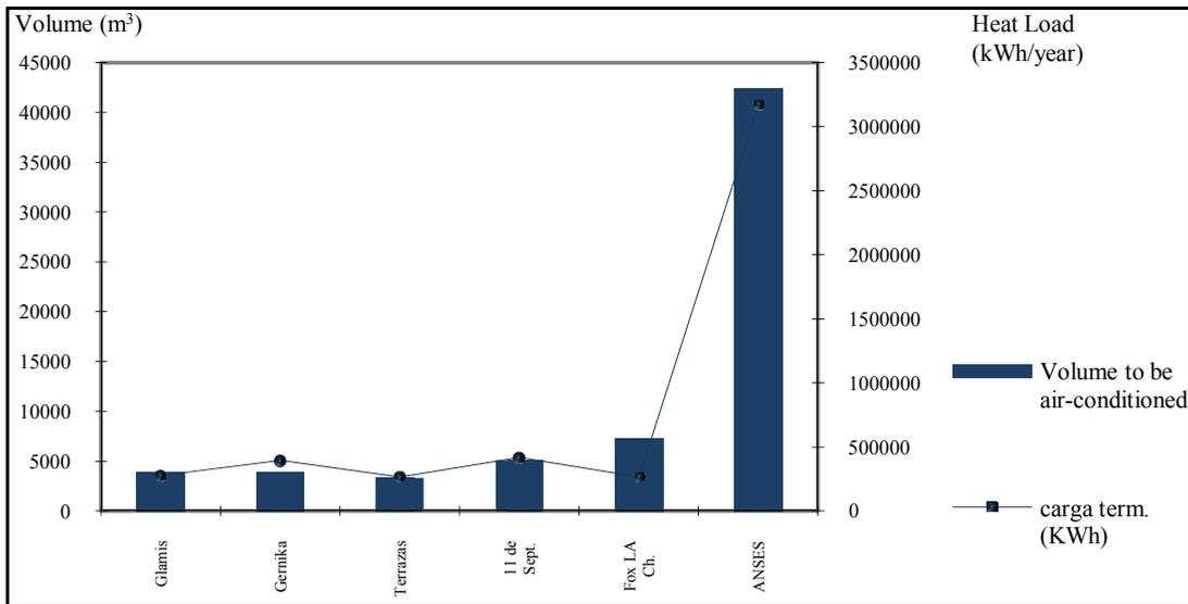
Figure 7. Relationship between the volume to be heated up/cooled and the heat load. Synthesis.
