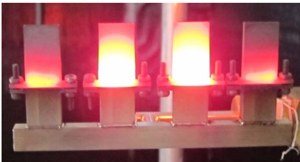
Figure 5. Experimental results showing the temperature distribution of single inlet pipe combustor.
