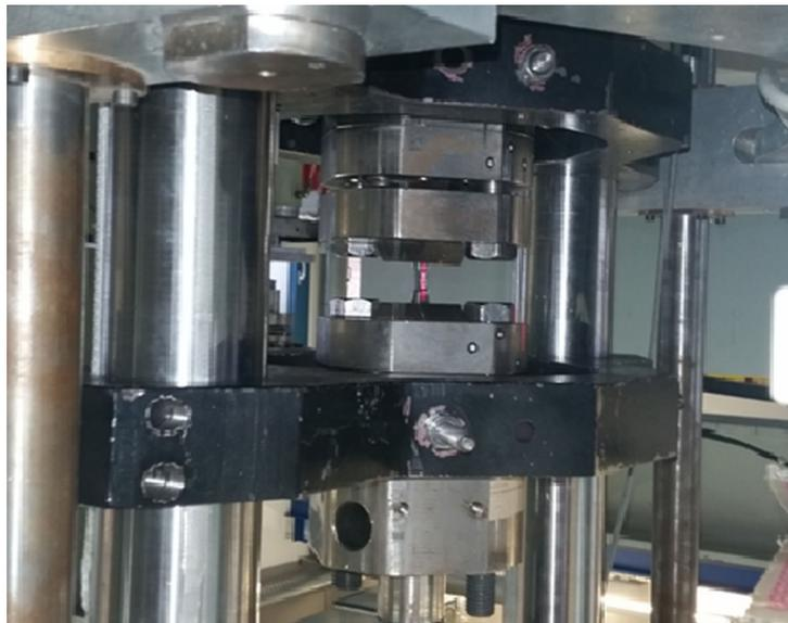
Figure 4. Tensile testing set up.
