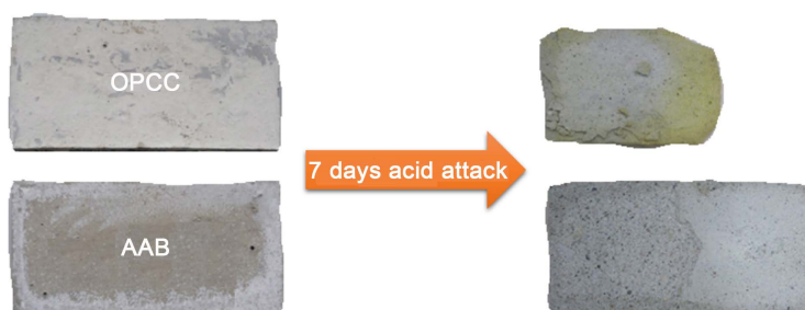
Figure 6. AAB and OPCC samples before (left) and after the acid attack (right).
