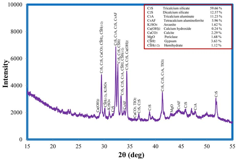
Figure 2. Mineralogical analysis of as-received cement using XRD.
