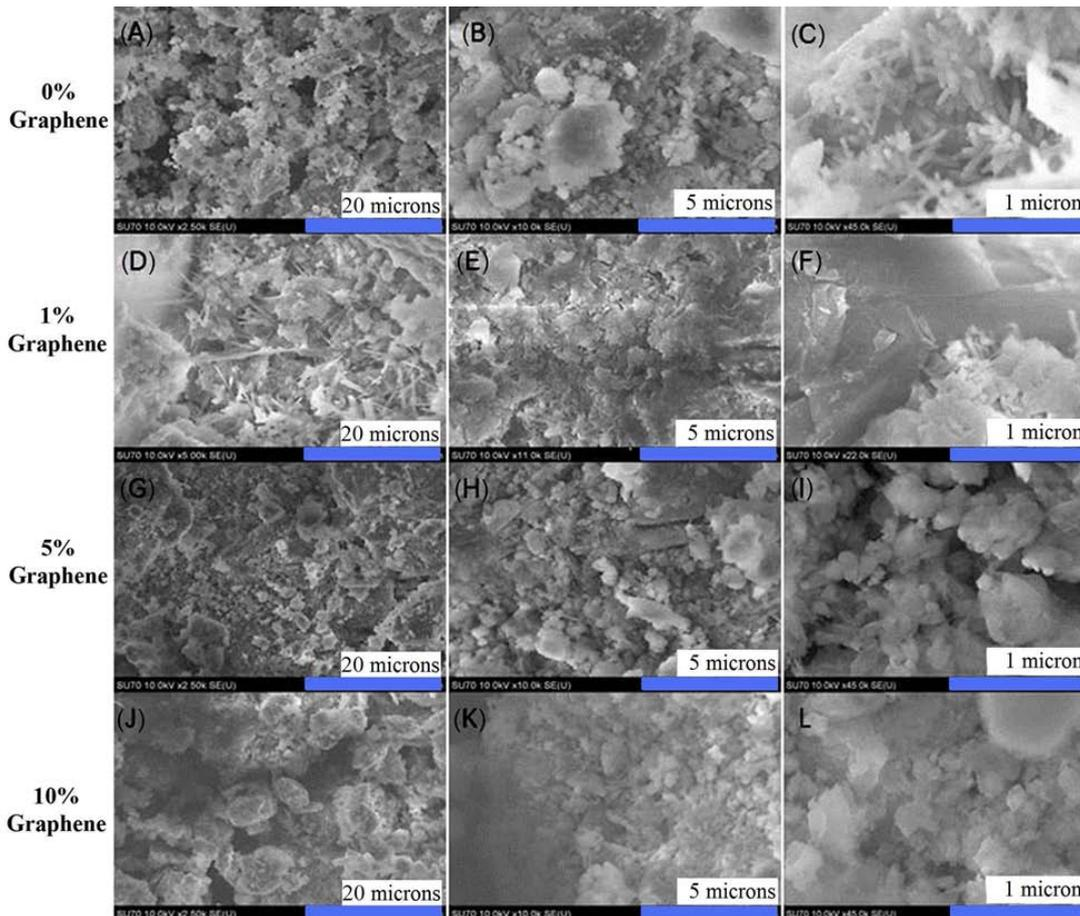
Figure 7. Scanning electron microscopy image of hydrated graphene-cement composite.
