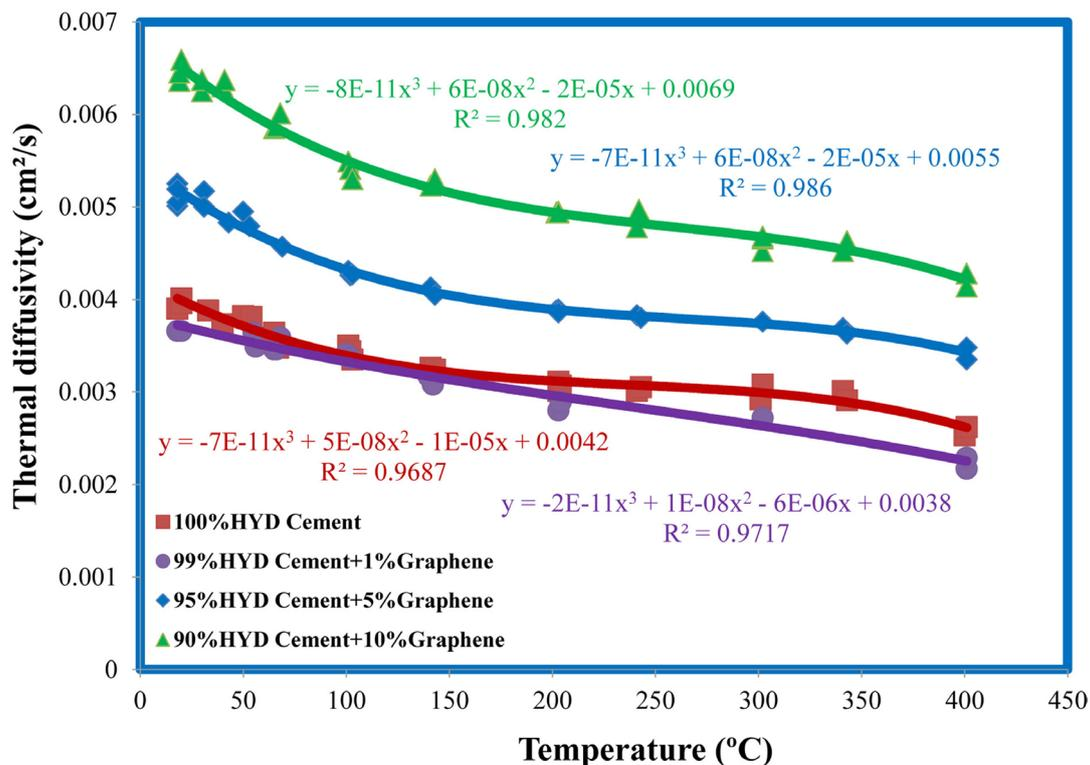
**Figure 9.** Thermal diffusivity of hydrated graphene-cement composites.
