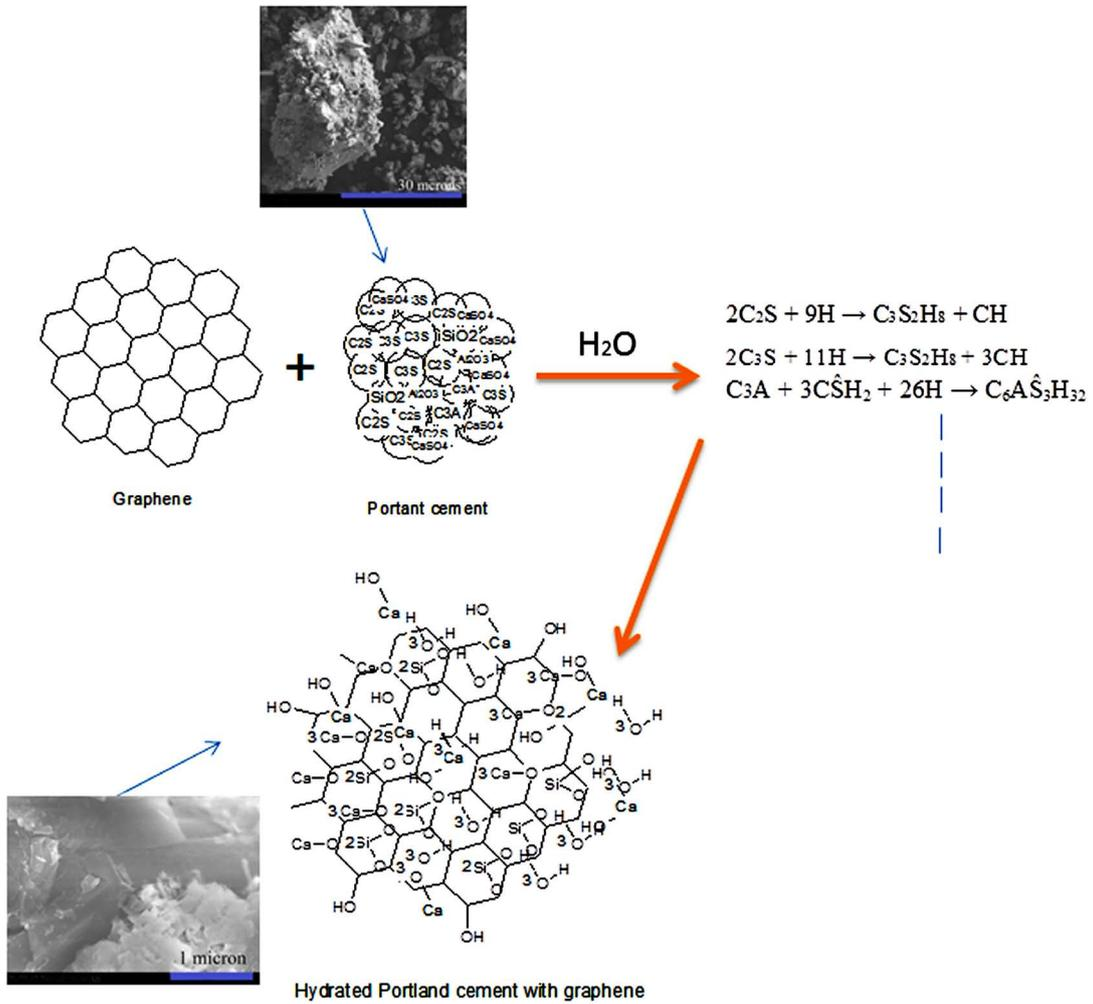
Figure 1. Schematic of hydrated graphene-cement composite and possible nanocomposite structure.
