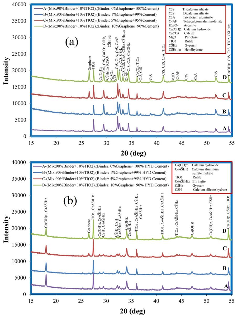
Figure 5. XRD patterns of cement & graphene-cement composites (a) anhydrous & (b) hydrated.
