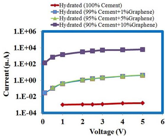
**Figure 8.** Electrical conductivity of hydrated graphene-cement composites.
