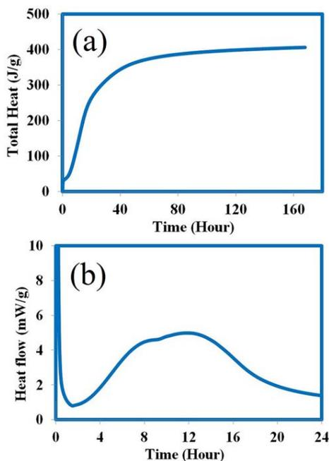
Figure 4. Cement paste (a) total heat & (b) heat flow.
