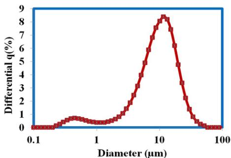
Figure 3. Particle size distribution of as-received cement.
