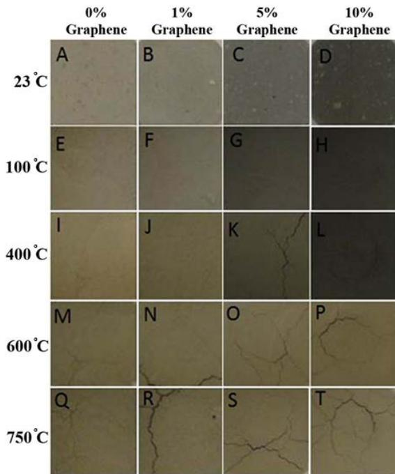
Figure 6. Temperature treatment of hydrated graphene-cement composites.
