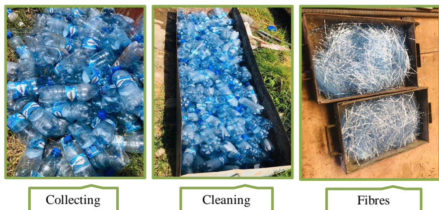
Figure 1. PET fibre preparation.
