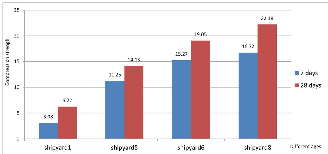
Figure 6. Resistance results of concretes to compression (two measures).
