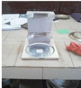
**Figure 2.** Surfacing square for concrete specimen, PROVITEQ type.
