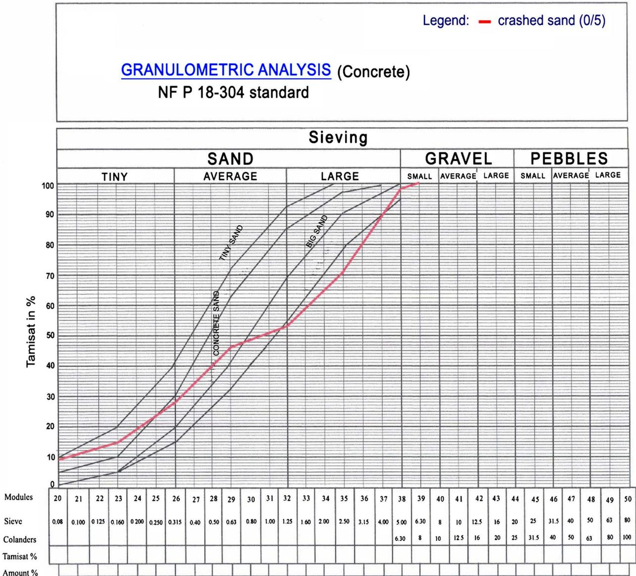
**Figure 8.** Particle size analysis of crushed sand.
