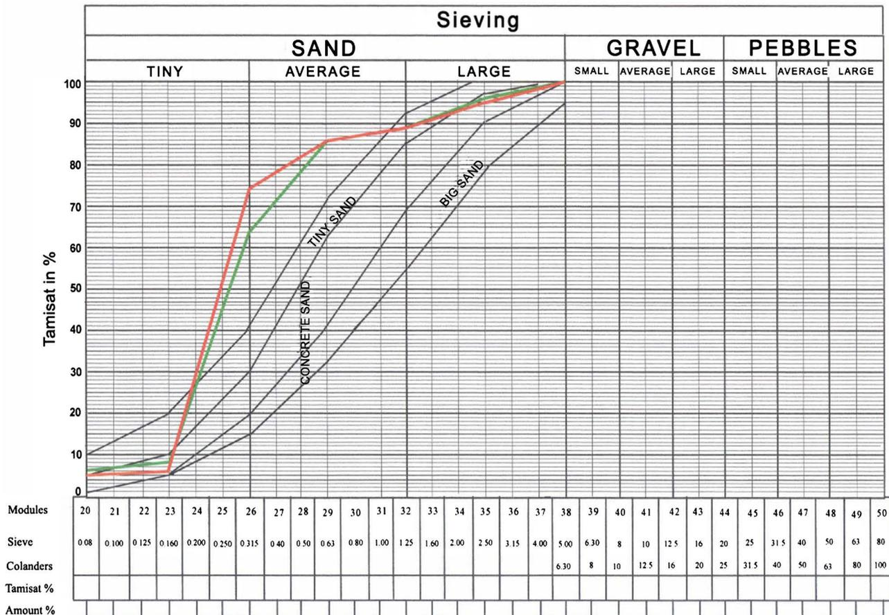
Figure 9. Particle size analysis of the improved Djiri and Congo River sands.
