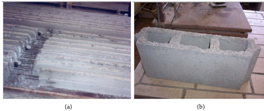
Figure 3. Prefabricated building elements. (a) Prestressed Beam create with the sand concrete; (b) Hollow bricks of concrete sand.
