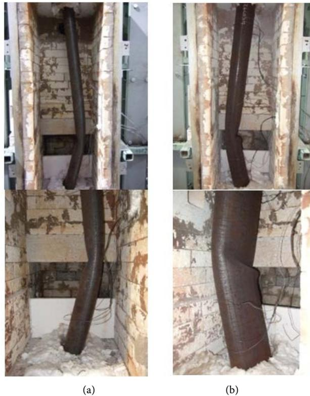
**Figure 7.** Failure modes of overall and local buckling of the elliptical hollow sections. (a) EHS-A (slenderness  $\lambda = 51$ ); (b) EHS-B (slenderness  $\lambda = 33$ ).
