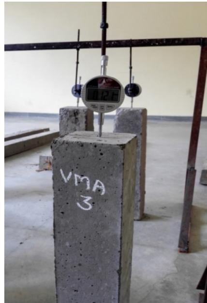
**Figure 1.** Shrinkage measurement.
