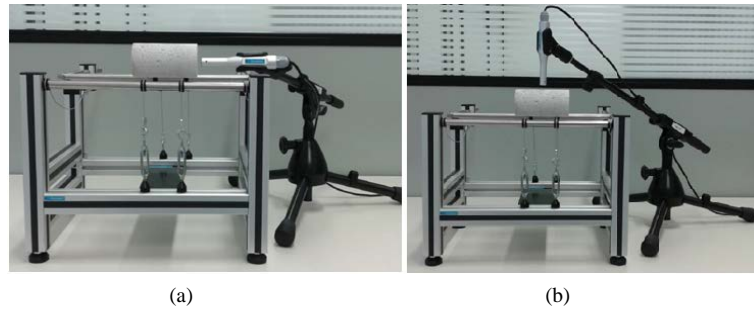
Figure 3. (a) Longitudinal ( E_{long} ); (b) Flexural ( E_{flex} ) Young's modulus.
