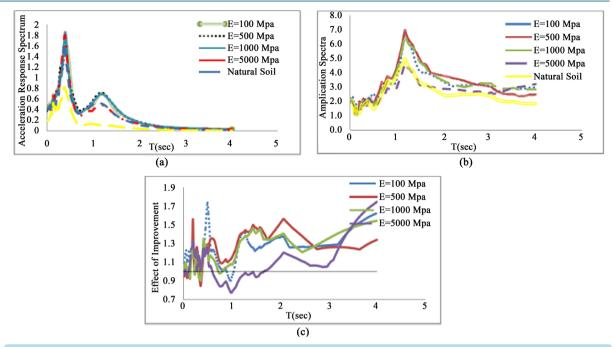
Figure 3. Comparison of seismic response on the surface of the natural ground and its improvement under near-fault Loma Prieta earthquake with PGA = 0.2 g: (a) elastic response spectra, (b) amplification of Sa, (c) the effect of improvement on Sa.
