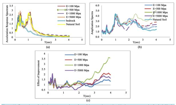
**Figure 10.** Comparison of seismic response on the surface of the natural ground and its improvement under far-fault Northridge earthquake with PGA = 0.7 g: (a) elastic response spectra, (b) amplification of Sa, (c) the effect of improvement on Sa.
