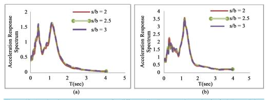
Figure 12. Acceleration response spectra for different pile distance ratios under far-fault Loma Prieta Earthquake with: (a) PGA = 0.2 g & (b) PGA = 0.7 g.
