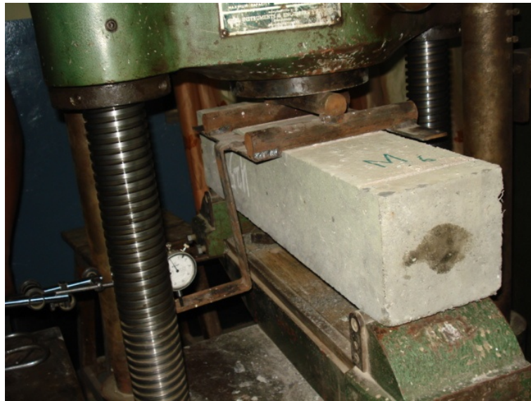
Figure 5. Flexure test on concrete beam under progress.
