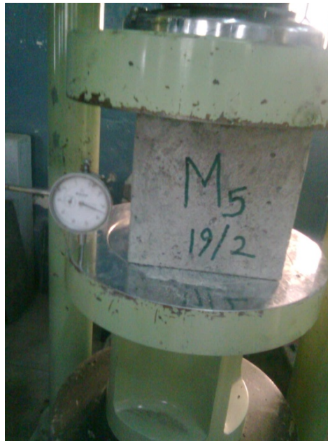
Figure 3. Compression test on concrete cube in progress.
