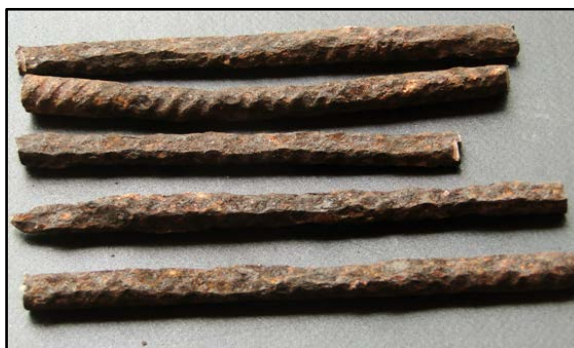
Figure 11. Carbon steel bars with localized corrosion.
