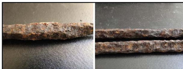
Figure 12. Carbon steel bars with localized corrosion.
