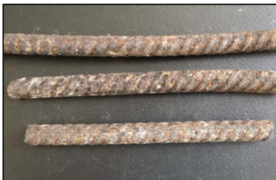
Figure 10. Carbon steel bars with uniform corrosion.
