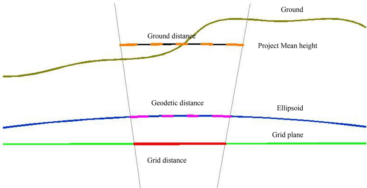
**Figure 2.** Grid and ground distances.
