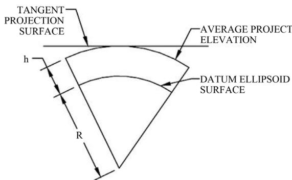
Figure 3. Tangent projection surface (after [16]).
