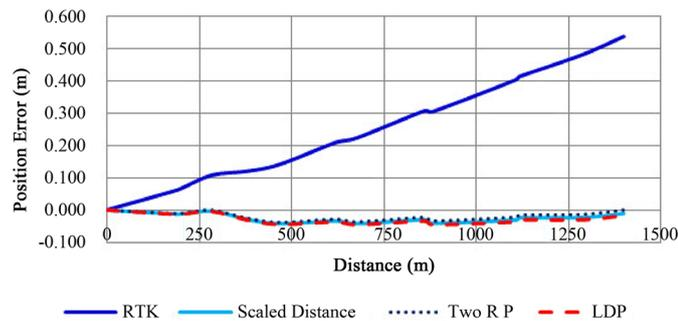
Figure 5. Error in relative position to the base point.
