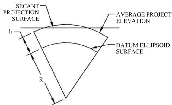
Figure 4. Secant projection surface (after [16]).
