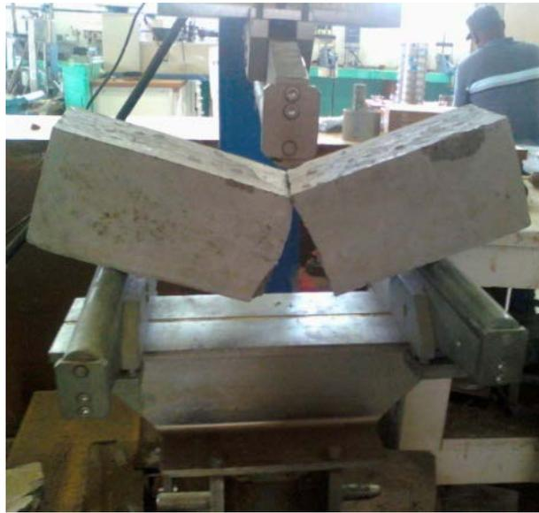
**Figure 2.** Typical flexural beam specimen failure.
