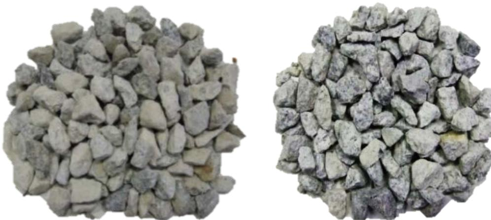
**Figure 1.** Batches of 19 mm recycled concrete and 19 mm natural aggregates.
