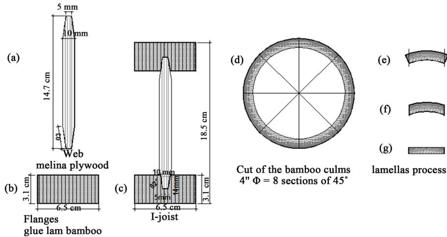
**Figure 1.** I-joists design (a), (b) and (c), lamellas obtained from the culms (c) to (g).
