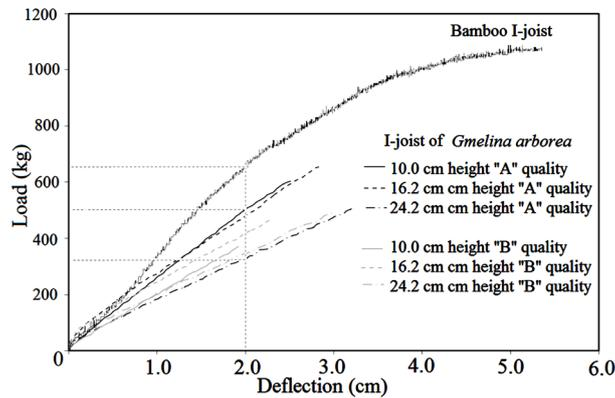
Figure 4. Comparison of the relationship between load vs. deflection for different types of I-joist used for *G. arborea* [4] and I-beams with bamboo flange.
