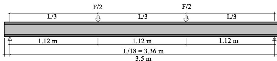
Figure 2. Loading arrangement for the flexure test.
