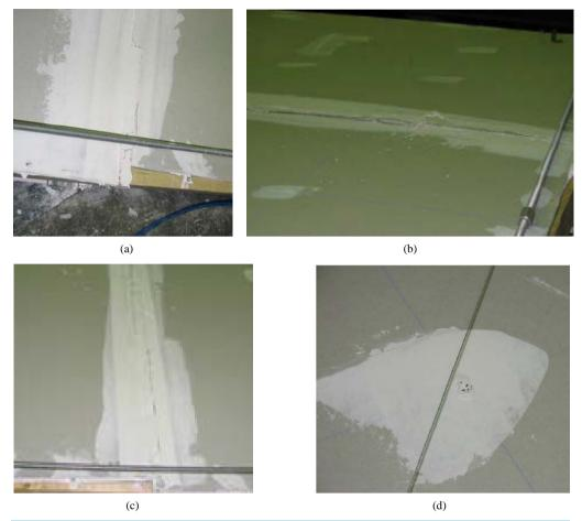
Figure 6. UGL specimen failure modes. (a) UGL edge tearout; (b) Relative movement of drywall; (c) UGL horizontal joint crack; (d) UGL screw attachment.
