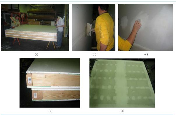
Figure 2. Construction and specimen details. (a) Attachment of sheathing; (b) Application of joint compound; (c) Finishing of joint compound; (d) Top and bottom plate; (e) Finished specimen.
