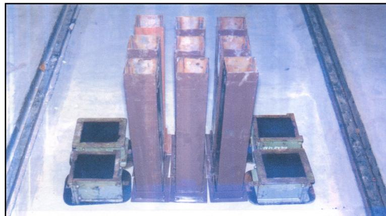
**Figure 2.** Steel box sections (100 mm × 100 mm × 750 mm) and standard mild steel mould.
