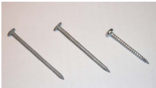
Figure 8. Left: annular nail; middle: smooth nail; right: screw utilized at non-yielding part of test-piece.
