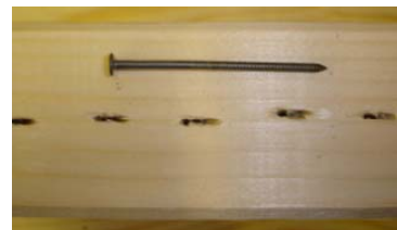
Figure 7. 10d spacing. No visible cracks.
