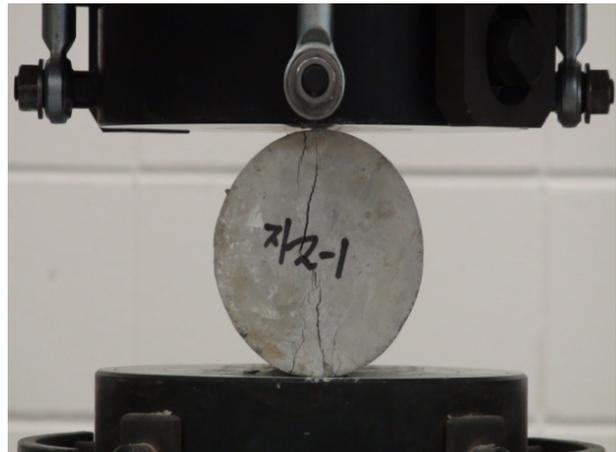
**Figure 4.** Splitting tensile strength test.
