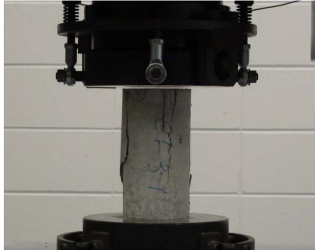
**Figure 3.** Compressive strength test.
