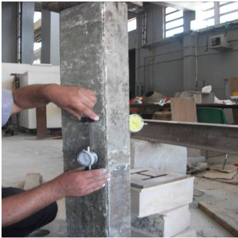
Figure 3. Composite basalt column under concentric load with strain and buckling (deflection) gages (transducers).
