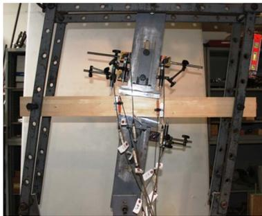
Figure 15. Continuous beam rotated by 0.005 rad.
