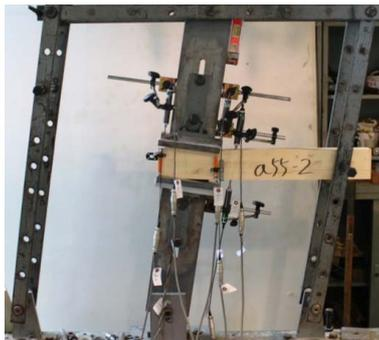
Figure 16. Cantilever beam rotated by 0.005 rad.
