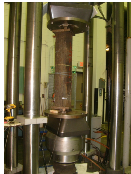
Figure 11. Installed specimen in the MTS testing machine.
