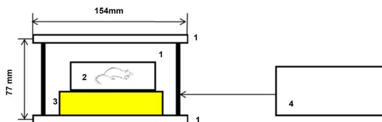
**Figure 1.** The exposure set up. 1—Helmholtz coil (D = 154 mm, H = 77 mm), 2—Plexiglas Box (134 mm × 105 mm × 55 mm), 3—Wooden table, 4—4 Hz and 8 Hz generator having output amplifier connected to coil.
