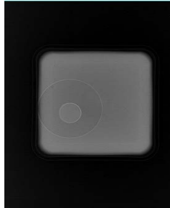
Figure 1. Film density of homogenous color (low contrast between the water and the palm leaves powder).
