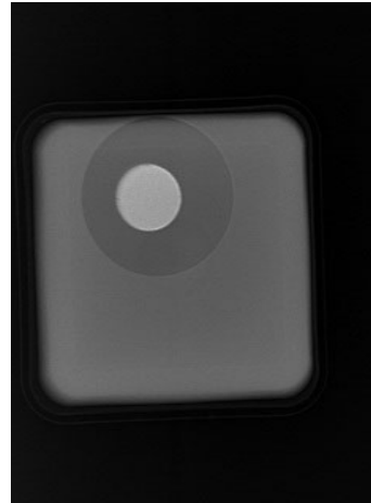
Figure 4. Petri dish on top of the water “PVC” of 1 cm showed very good concentration “film density” as skull bone. It is the densest material of the experiment.
