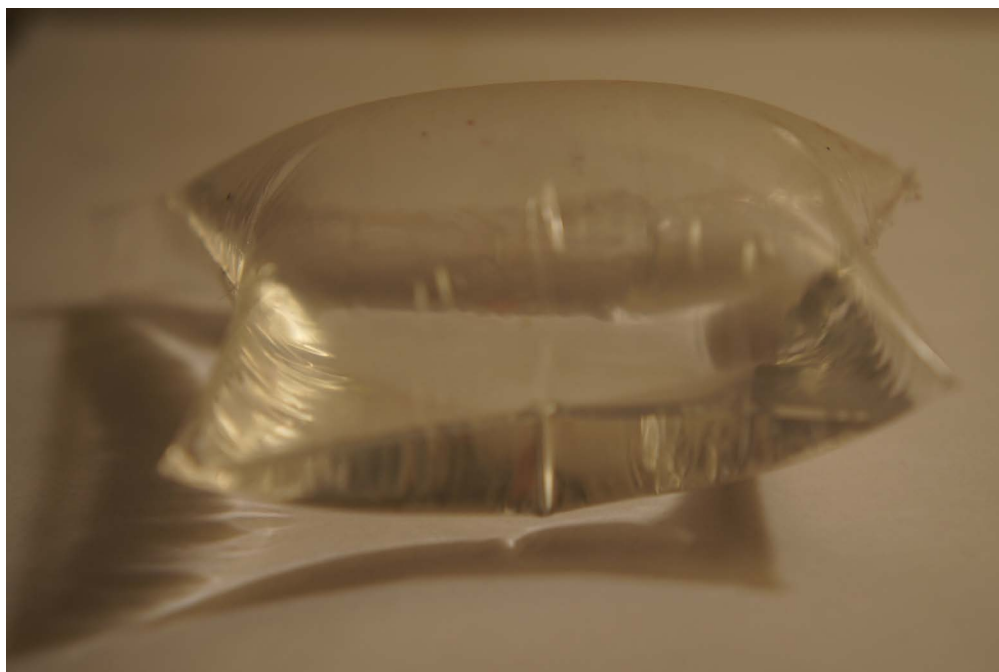
Figure 3. An expanded portion of a Ziploc™ bag that was heat-sealed after adding approximately 30 ml of activated ethanol. The ethanol had been activated by prior condensing ethanol vapor onto a dome of a running Van de Graaff generator. As in the example shown in Figure 1 , the container was initially flaccid but by about a month began to expand. By 3 months, the container was markedly expanded and has remained so for over 2 years with gradually reducing amount of fluid.
