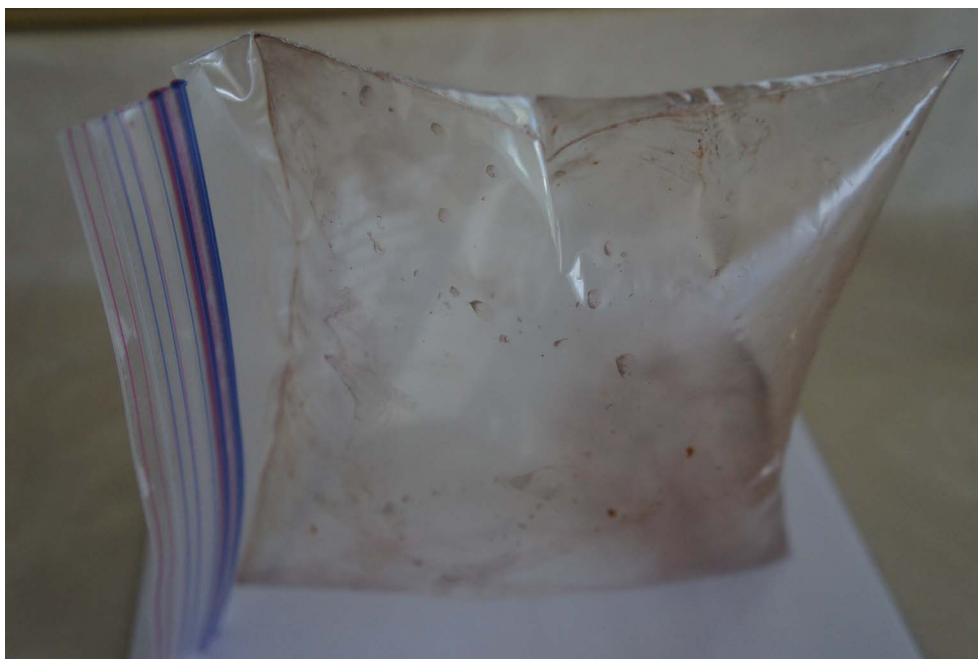
Figure 2. Photograph of an expanded Ziploc™ bag. Approximately 30 ml of activated ethanol plus neutral red dye had previously been added to the bag, which was then heat sealed just below the interlocking closure. The bag underwent considerable expansion while retaining much of the original solution. The amount of fluid slowly diminished over approximately a year, leaving a still expanded bag with no residual fluid. The fluid-less bag has remained expanded for more than 2 years, with a gradual reduction in volume.
