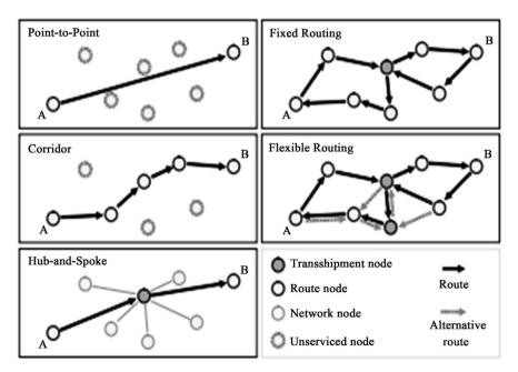
**Figure 4.** Freight distribution systems Source: The transport geography of logistics and freight distribution.
