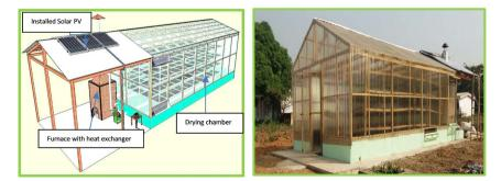
Figure 1. Solar Biomass Hybrid Dryer; schematic view (left) and constructed view (right).
