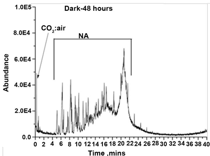
**Figure 5.** GC-MS analysis of head-space aliquots from UV photocatalysis of naphthenic acid by of Z-TiO<sub>2</sub> after 48 hours. Adapted from (Kalebaila and Fairbridge, 2014).
