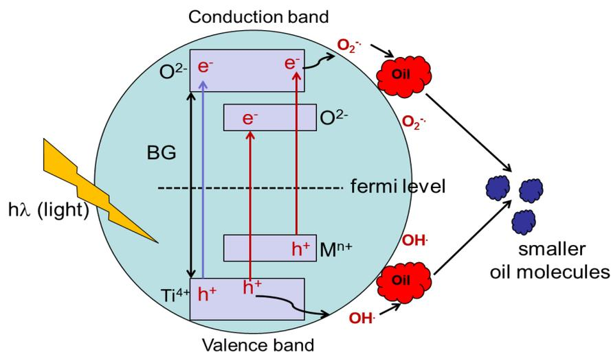
**Figure 4.** Adsorption and decomposition of organic molecules on  $\text{TiO}_2$  photocatalyst by radicals.
