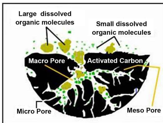
**Figure 2.** Physical morphology of activated carbon matrix. Source: <http://biomassproject.blogspot.com/2017/02/activated-carbon-production-from.html>.
