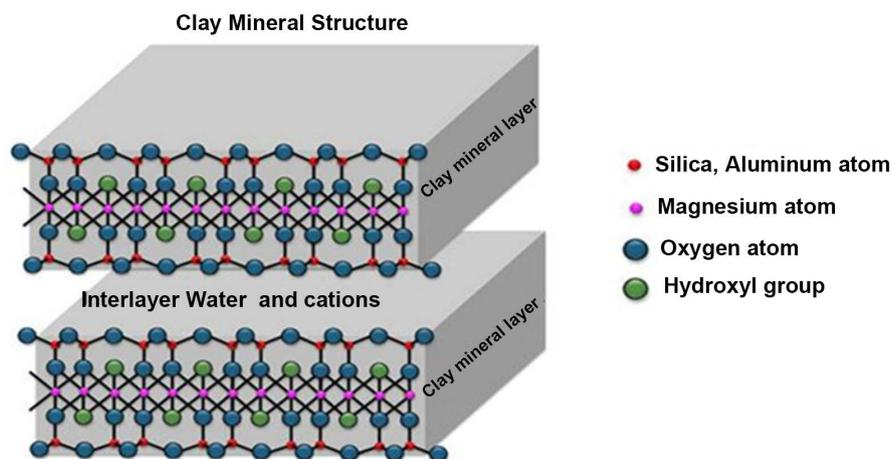
**Figure 3.** Typical structure of natural clay (image adapted from <https://www.jpl.nasa.gov/spaceimages/details.php?id=PIA17598>).
