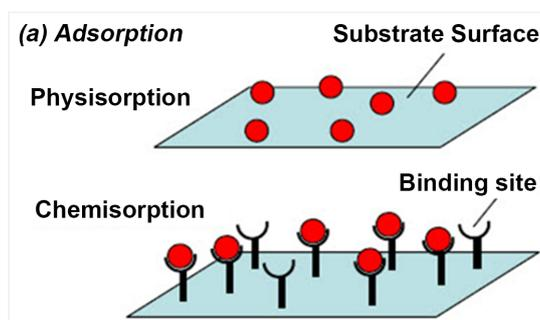
**Figure 1.** (a) Depiction of physisorption and chemisorption interaction between the substrate surface (adsorbent) and the adsorbate molecules (Adapted from <https://hub.globalccsinstitute.com/publications/co2-capture-technologies-post-combustion-capture-pcc/adsorption>).
