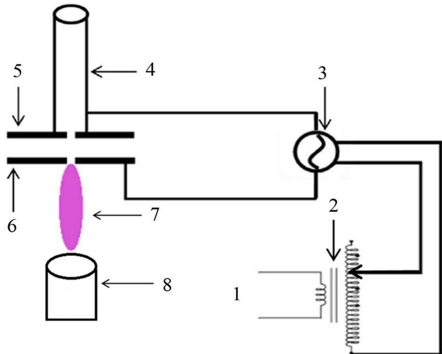
**Figure 1.** The electric circuit of cold atmospheric plasma jet device, 1 input electric source 220 V, 2 voltage controllers, 3 neon power supply, 4 gas feeding through copper tube, 5 anode, 6 cathode, 7 plasma jet and 8 acrylic box.
