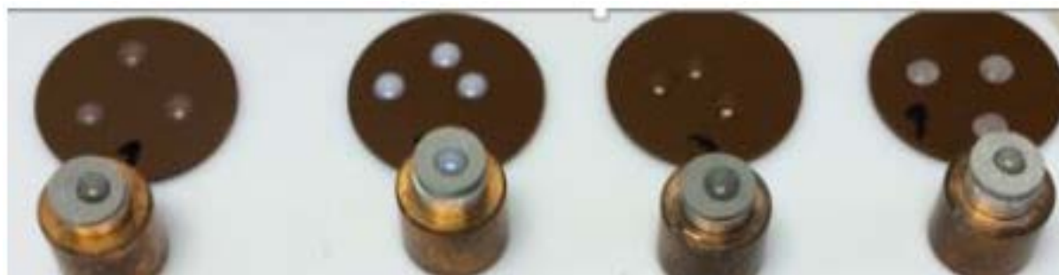
Figure 7. Wetting probes on polyamide and titanium. From left to right: Pearlbond DIPP 539, Griltex D1582E, Lotryl 35BA320, Capa 6250.
