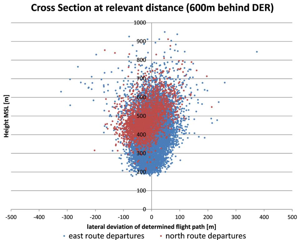
Figure 14. Relevant cross section passing through the critical obstacle at 600 m DER distance, departures from runway 07C.
