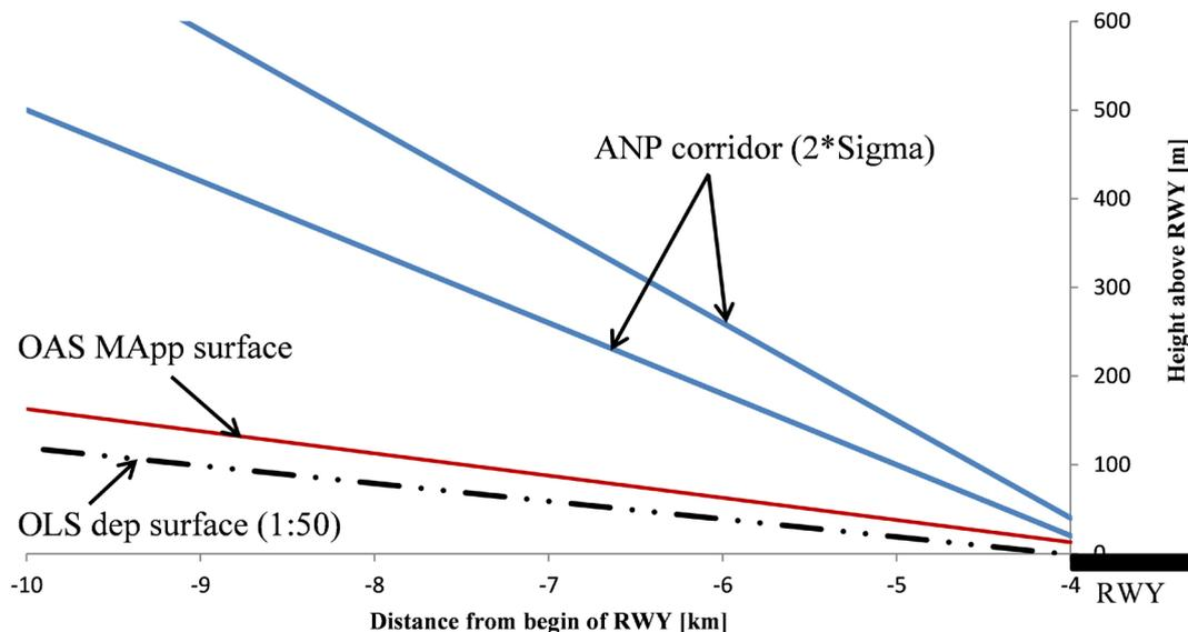
Figure 3. Heterogeneous safety margins resulting from OLS and OAS (departure).
