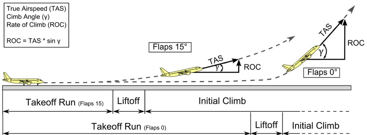
**Figure 10.** Lowest pass altitude analysis for take-off obstacle clearance.
