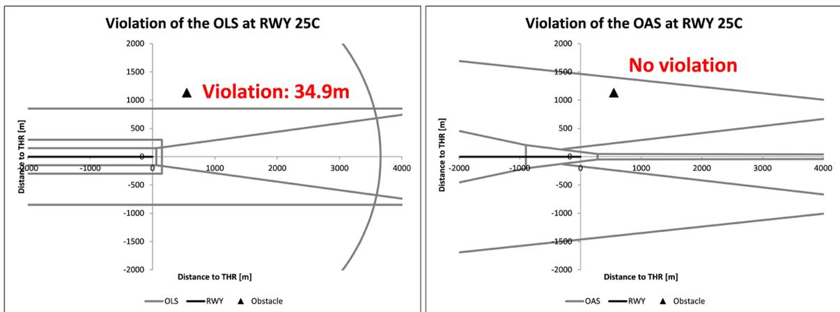
Figure 12. Excerpt of the obstacle clearance analysis for the runway 07/25C, OLS—left figure, OAS CAT I—right figure.
