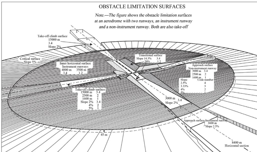
Figure 1. Obstacle limitation surfaces, Annex 14, Att. B; p. 313 [1].
