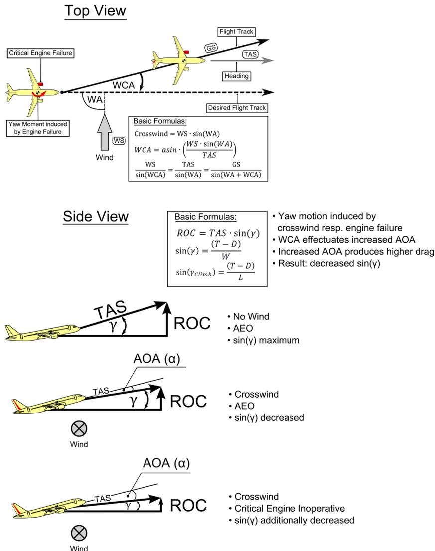
**Figure 8.** Underlying flight performance in the DOM. AOA = angle of attack, WA/WS = wind angle/speed, AEO = all engines operative.
