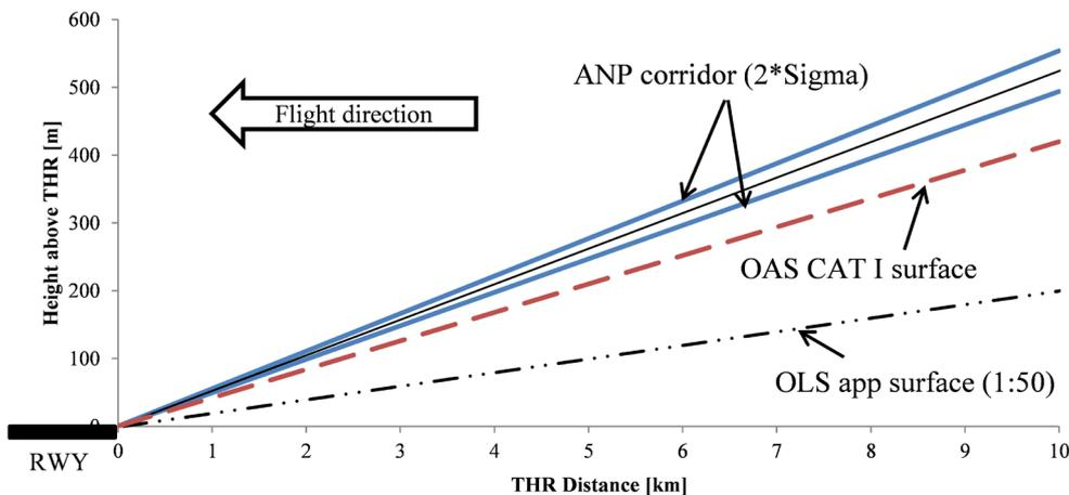
Figure 2. Heterogeneous safety margins resulting from OLS and OAS (during approach).
