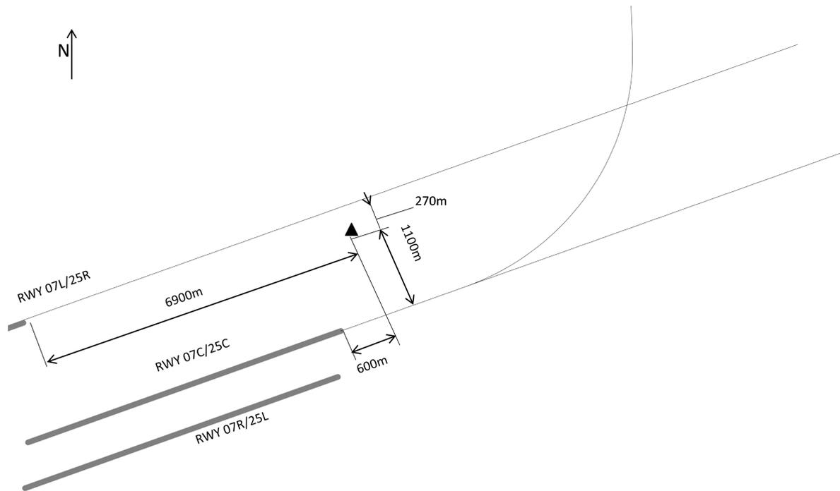
Figure 11. Location of the critical obstacle—the safety case EDDF.
