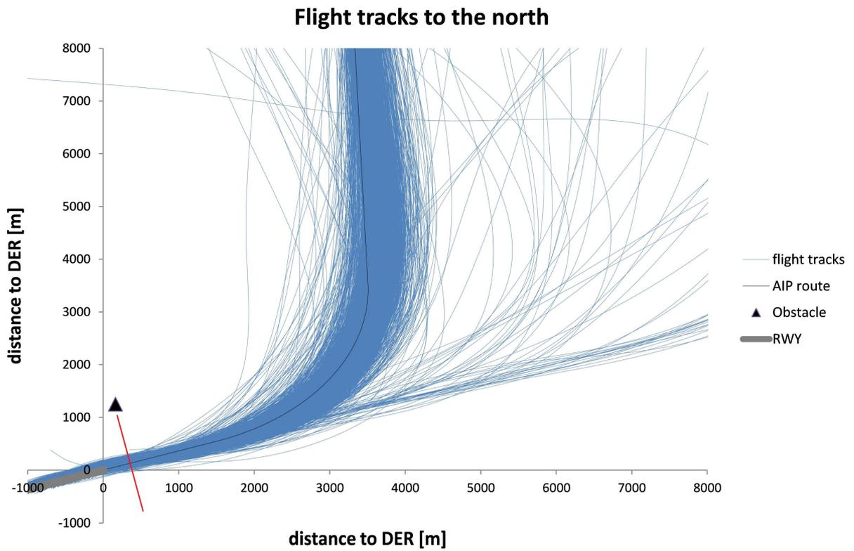
Figure 13. FRA Flight tracks for runways in use 07, outbound flights, FANOMOS Data, with obstacle critical cross section (red line).
