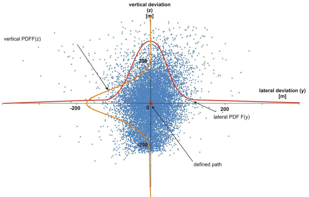
Figure 6. Normally distributed track offsets around the flight path.
