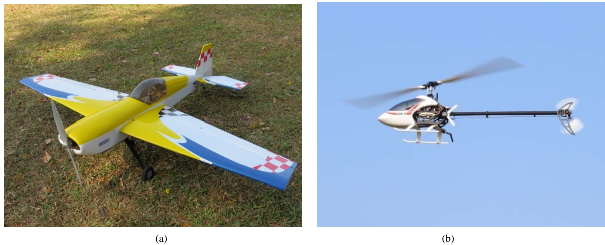
Figure 2. RC model aircraft employed in this study: (a) 25% scale Extra 260; (b) Logo-10 with stretched tail-boom to accept 600 mm main blades.
