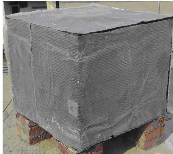
Figure 1. Front view of the integrated collector storage solar water heater.
