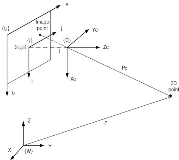
**Figure 1. Pin-hole camera model.**
