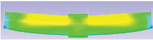
Figure 3 Strain distribution and deformation (Scale factor: 1 \times 10^5 )
