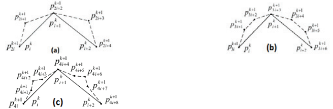
Figure 1: (a), (b) and (c) represent binary, ternary and quaternary refinement of coarse polygons using (1) for n = 2, 3, 4 , respectively.
