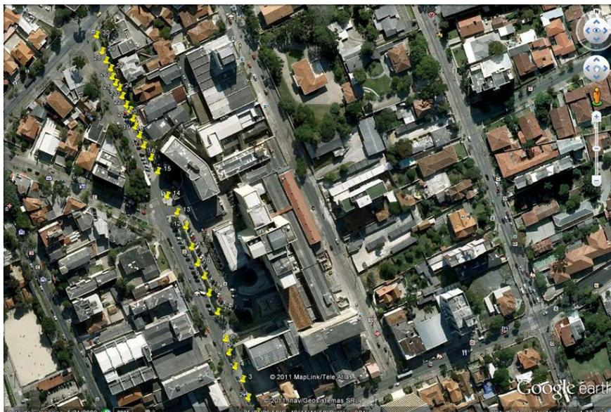
**Figure 1.** Noise measurement points along the frontal façades of the buildings of the University Hospital of the Federal University of Paraná—UFPR.
