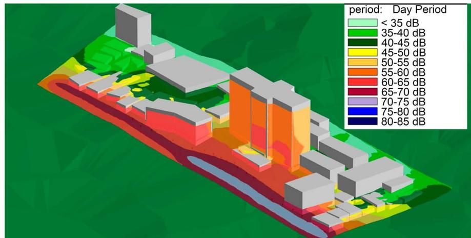
**Figure 4.** Three-dimensional noise mapping of the frontal façades of the buildings of the University Hospital of the Federal University of Paraná—UFPR.
