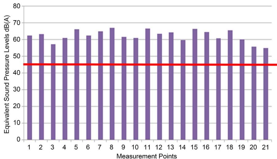
**Figure 6.** Comparison of measured indoor sound pressure levels with the limits established by standard NBR 10152:87.
