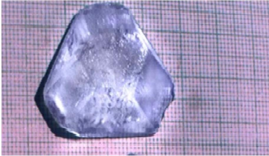
**Figure 1.** Grown crystal of Lithium Sodium Sulphate Hexahydrate (LSSW).
