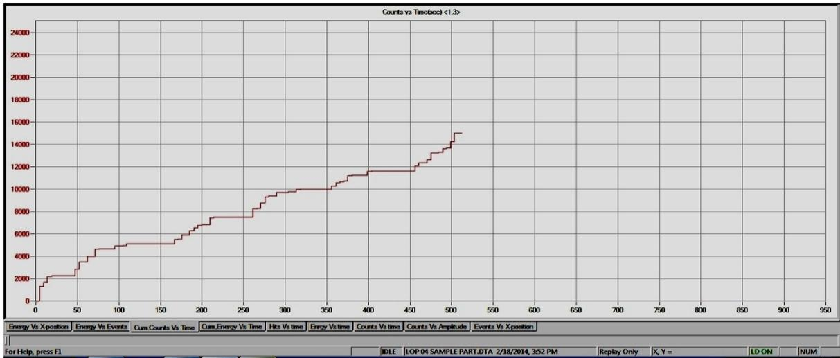
Figure 11. Cumulative Counts vs. Time for Lack of penetration defect of SS316L.
