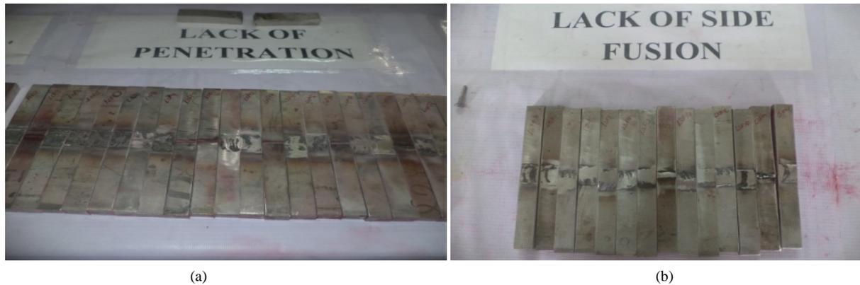
**Figure 7.** SS316L samples containing (a) Lack of penetration; (b) lack of side fusion for AE study under constant load.
