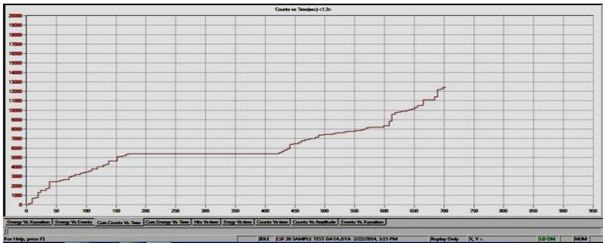
Figure 12. Cumulative Counts vs. Time for Lack of side fusion defect of SS316L.
