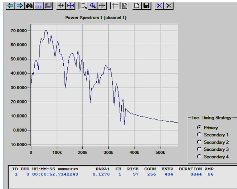
Figure 25. Frequency Spectrum for Lack of penetration defect of SS316L.
