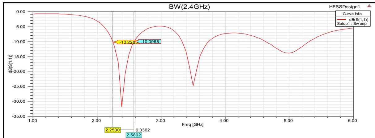
Figure 7. Simulated Bandwidth of the Monopole Antenna resonating at 2.4 GHz indicating a Bandwidth of 330.2 MHz.
