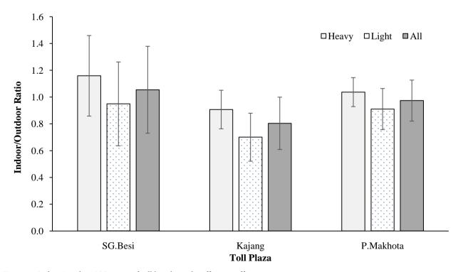
**Figure 4.** Indoor/outdoor NO<sub>2</sub> ratio of toll booths and traffic type effect.
