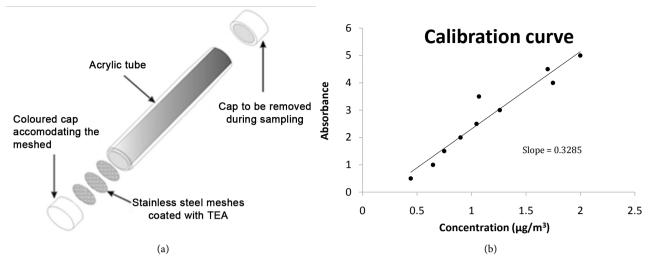
Figure 1. (a) Schematic of NOx diffusion tubes; (b) Calibration curve.
